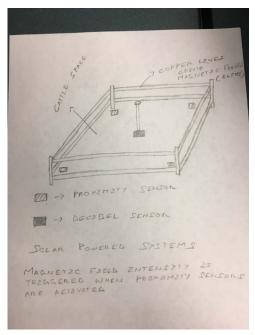
The decibel sensor allows the farmer to monitor any unexpected or violent behavior of the cattle by sensing the frequency variation of the cattle's voice or cow bell. The threshold of the decibel sensor is set in such a way that whenever the cow pitch/vibration of the cow bell exceed its normal day to day pitch/vibration level, the sensor gives an alert. The sensor can also be used to monitor cattle's health.
