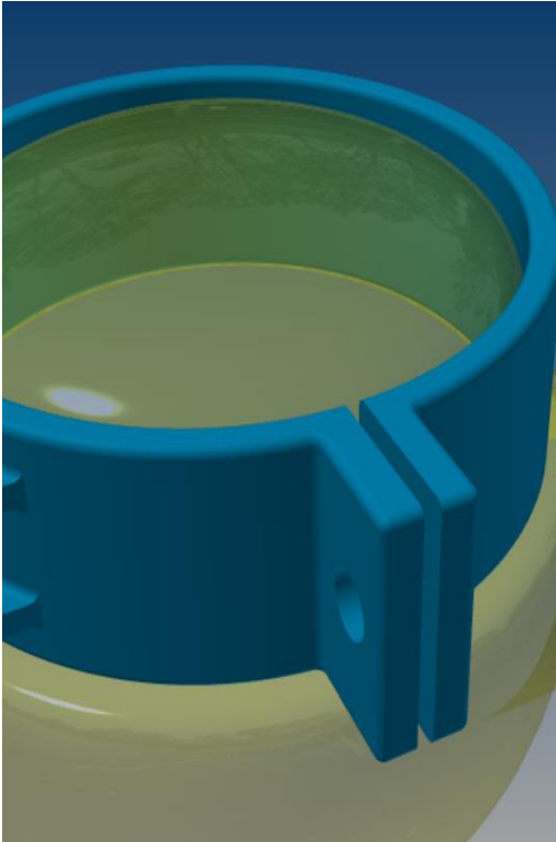
Figure 7: Clamp Design Requiring Ductile Material Properties
