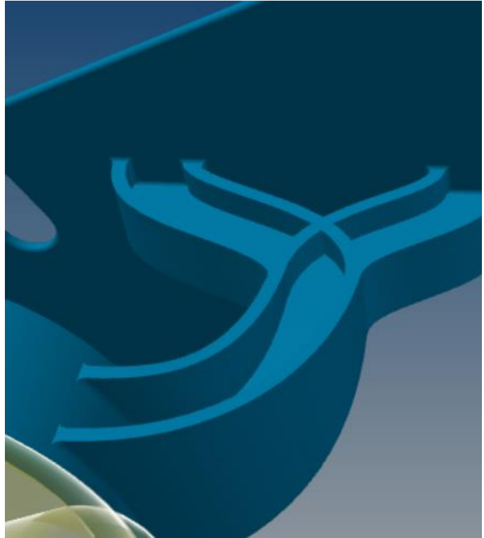
Figure 8: "I-beam" Design for Increased Rigidity
